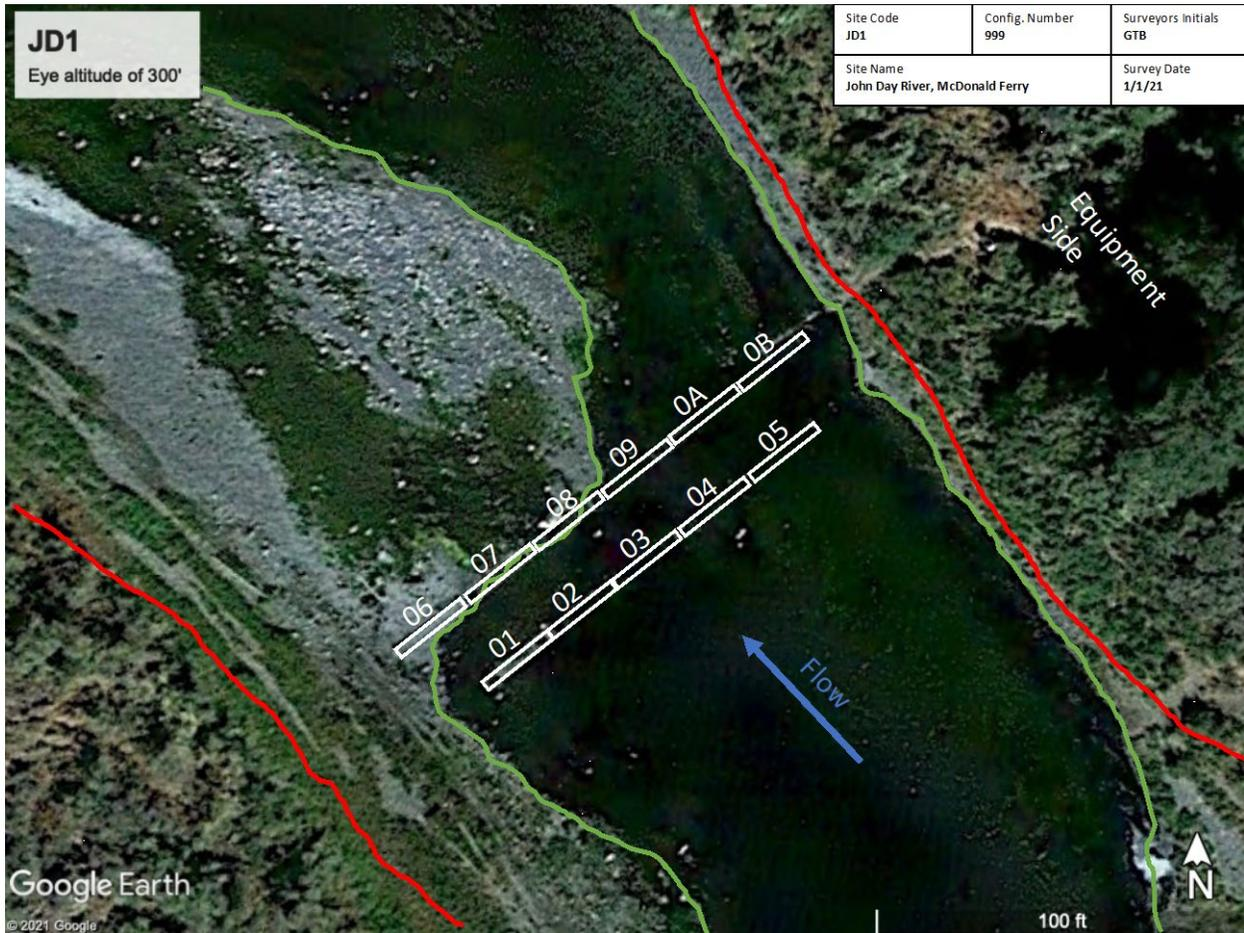
Figure 8. JD1 with direction of flow, antennas, and approximate high and low water lines completed.
